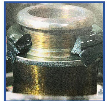
Bad oil rail seal
